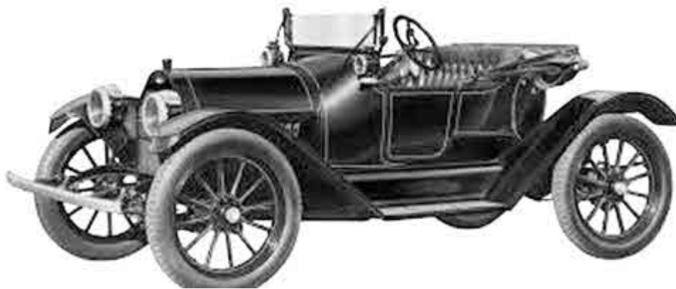
Photo: The 1916 Chevrolet 490 came in a touring car and a roadster model. Competing with the Ford Model T, it had a 171 cubic inch engine with a three-speed transmission and like the Model T it was only available in black.
