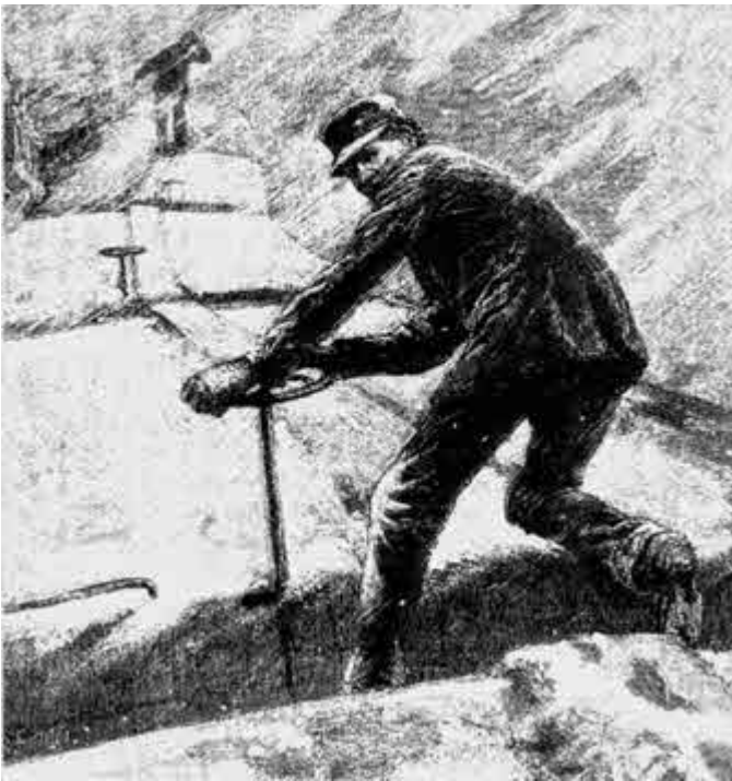
A brakeman's job was dangerous and involved running atop the train cars in many kinds of weather to set the brakes.
