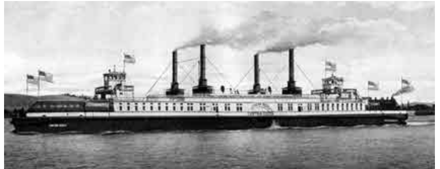
Ferry Boat carrying the train: Look closely and one can see the specially made ferry boat that was designed to carry the train across the Carquinez Straits. Circa 1910.
